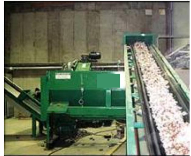
In the Air Classifier Module, material is sorted by an air knife. The heavier material drops into the Heavy Fractions discharge conveyor. This material consists of organics, shoes, wood, and heavy non-ferrous metals. These are hand sorted to remove non compatibles, the remaining combustibles are returned down stream of the Eddy Current Separator (ECS).
